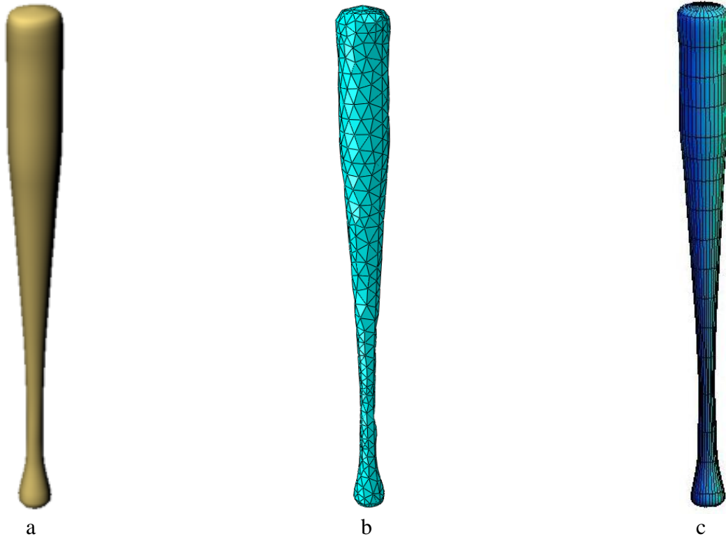
Figure 8. A geometric comparison of a baseball bat model (a) Rhinoceros CAD software (b) ABAQUS FEA analysis program (c) Mathematica tensor-product analysis code
